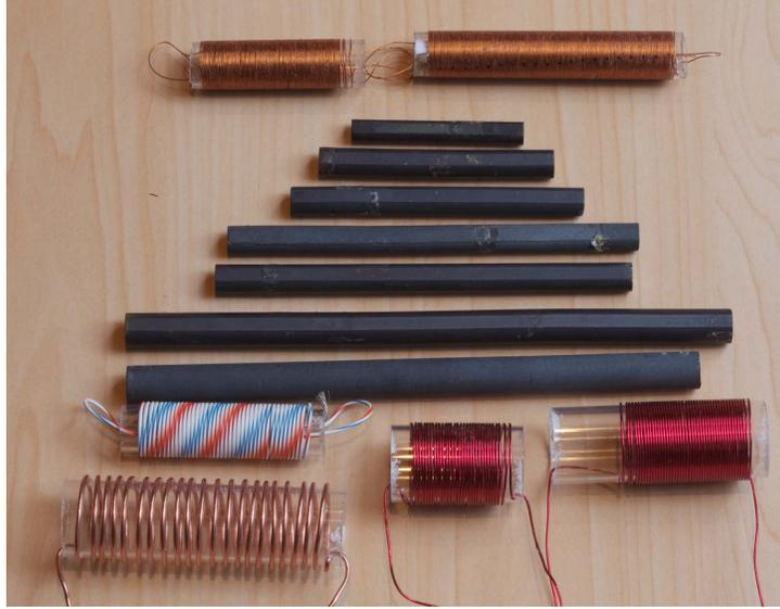
Figure 5: Some of the rods and coils tested
